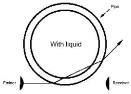
If the diameter of the pipe is close to 6 mm, some of the emitted light may reach the receiver because the angle of refraction is small. This may result in false readings. In such cases, set the sensitivity selector to Low and check that the EE-SPX613 reads correctly for pipes with and without liquid.
